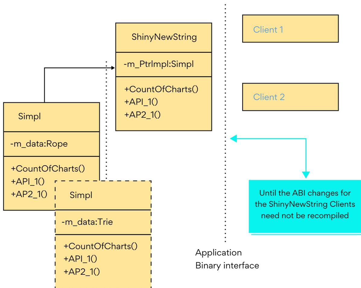
Since the design uses a pointer to implementation, changes to internal implementation are opaque to external clients of the class. This is exactly why the technique is also known as compile-time firewall.
