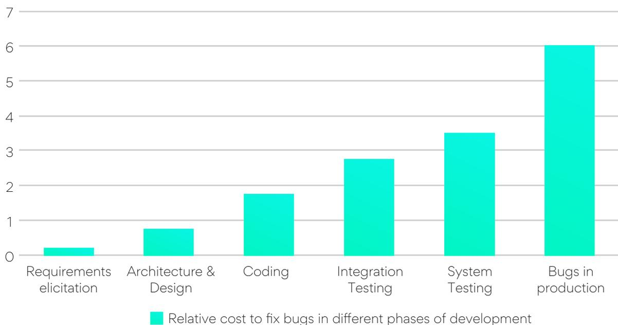
This is a well-known graph of relative cost to fix bugs based on the time of detection. If testing suffers due to longer build times, it is natural that more and more bugs will escape undetected to production. This will increase the overall cost of development and the quality of the software will suffer. In the current fiercely competitive market, top-quality frequent releases are vital.
