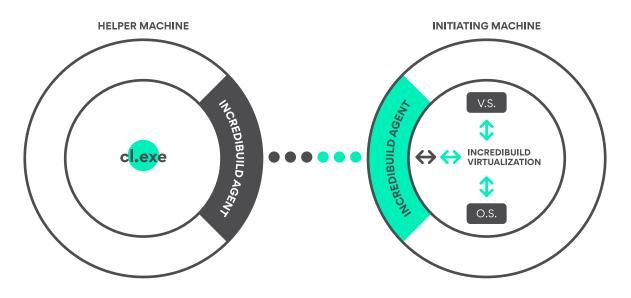
**10.** When the Incredibuild Agent on the remote machine executes the compilation process, the virtualization layer is once again injected into the process (cl.exe). It intercepts all calls that the cl.exe process sends to the OS.
