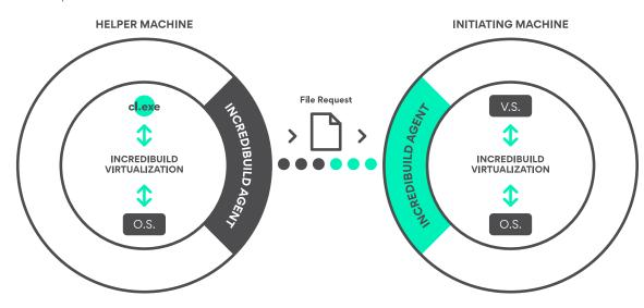
**13.** The requested file is copied from the local host machine's file system to an Incredibuild cache folder on the remote machine.
