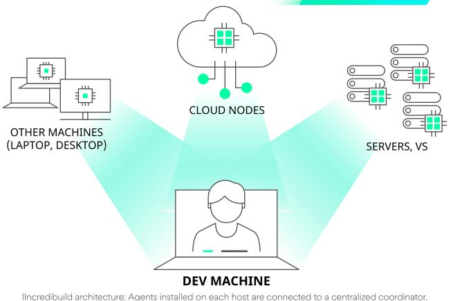
Incredibuild architecture: Agents installed on each host are connected to a centralized coordinator. Each host machine with an agent can use the aggregated idle power of all the other machines in the Incredibuild environment.
