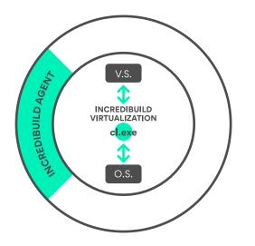
4. Incredibuild detects cl.exe as a process predefined to run on remote machines if possible, and does not allow the request to create the compilation process to reach the operating system.
