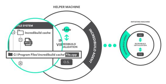
**15.** The operating system locates the file in the Incredibuild cache folder, opens it, and returns a file handle to Incredibuild, which forwards it to the compiler process. The result: The OS opens a valid file, the compilation process receives a valid handle for the file it requested, and the compilation process continues – all while Incredibuild continues to emulate the local machine's environment.
