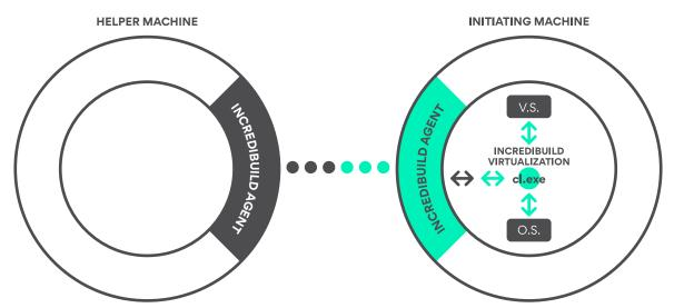
8. Once the Incredibuild Agent on the local host machine gets a remote machine on which it can execute the compilation process, Incredibuild informs Visual Studio that the compilation process it requested was executed. Yet, instead of a handle to the real process, Incredibuild returns a dummy process handle to Visual Studio. Visual Studio now understands that a compilation process is running on the local host machine.
